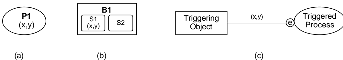
Figure 2: Expression of temporal constraints in OPDs. (a) process duration constraint; (b) state duration constraint; (c) reaction time constraint.
