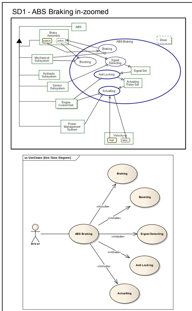
Figure 4. Example of Use Case Diagram generation ( $k=2$ )
